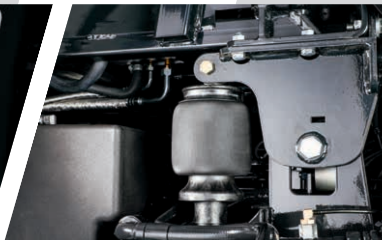
> Pneumatic cab suspension for a smoother ride.
