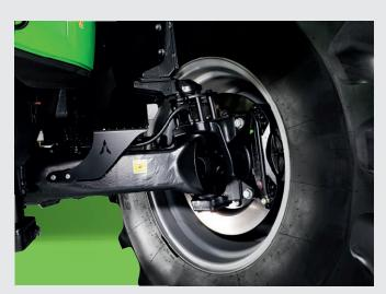
⚠ Dry disc brakes for maximum brake performance.
