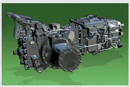
↑ SDF T7780 TTV compound transmission.
