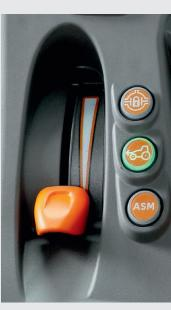
★ Electro hydraulically operated 4WD and differential lock including ASM.
