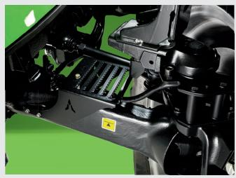
Maintenance steps above the front axle for comfortable cleaning.
