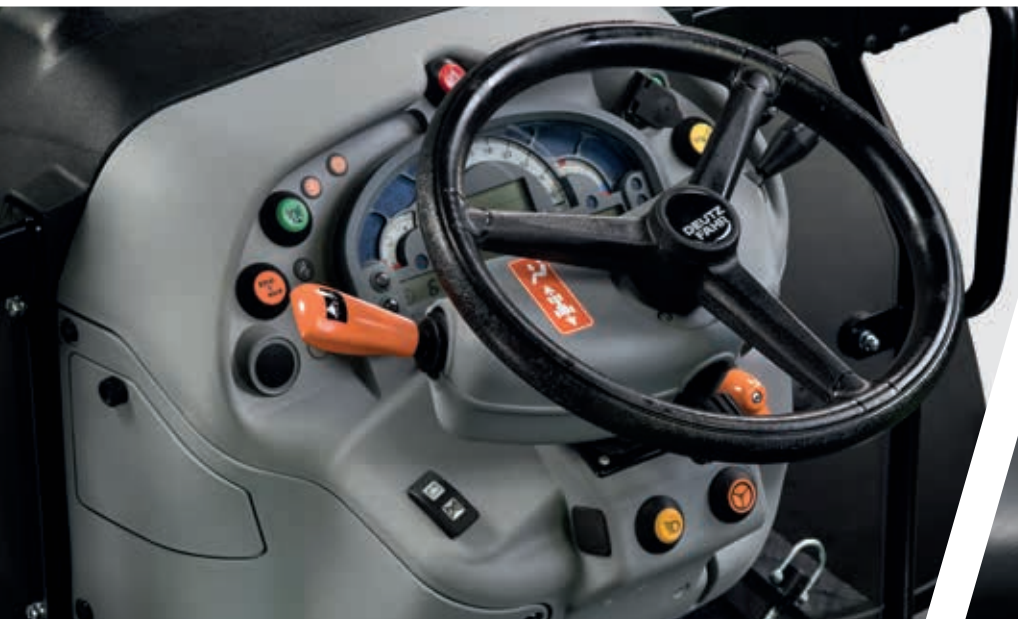
> PowerShuttle with Stop&Go function.
