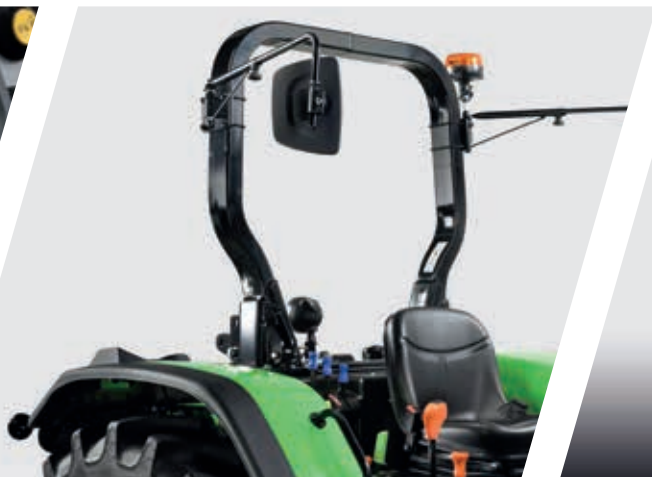
> Rear mirrors installed on ROPS.
