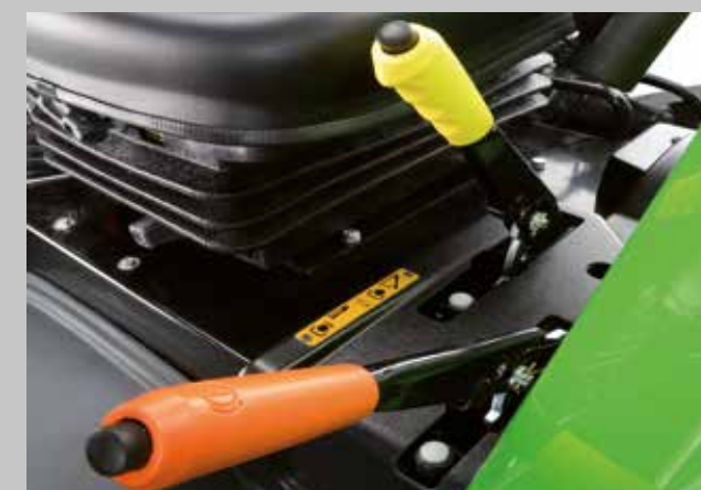
Parking brake and PTO controls are within easy reach on the left.
