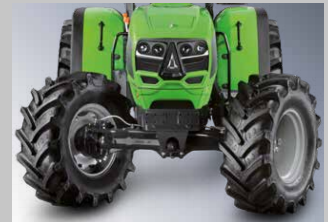
The compact bonnet allows a steering angle of up to 55°.
