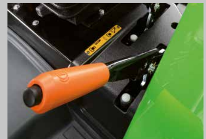
Mechanical parking brake installed beside the driver's seat within easy reach.
