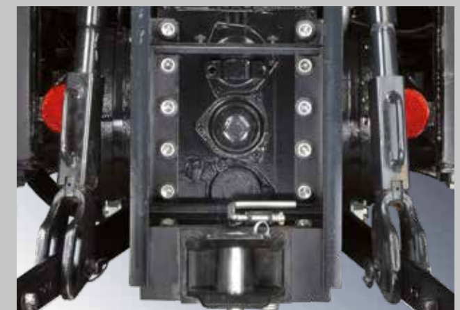
PTO: 540 or 540/540ECO or 540/540ECO/1000 or 540/540ECO plus ground-speed PTO can be selected.
