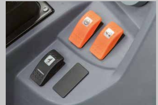
Option of mechanical or electro-hydraulic activation of the four-wheel drive and differential lock.
