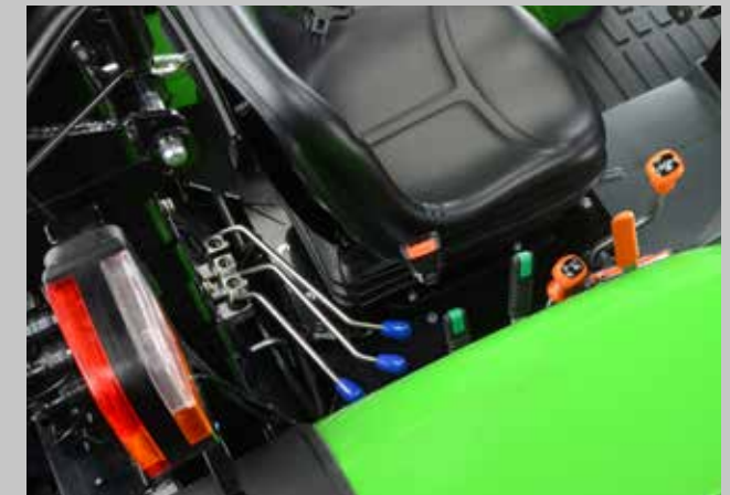
Up to three mechanical control units in the rear.
