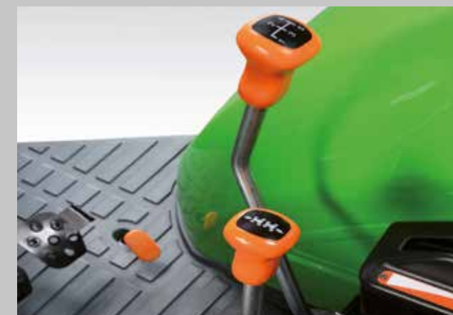
Transmission controls, manual throttle, engine speed settings, rear power lift and hydraulic controls are within easy reach on the right of the driver.
