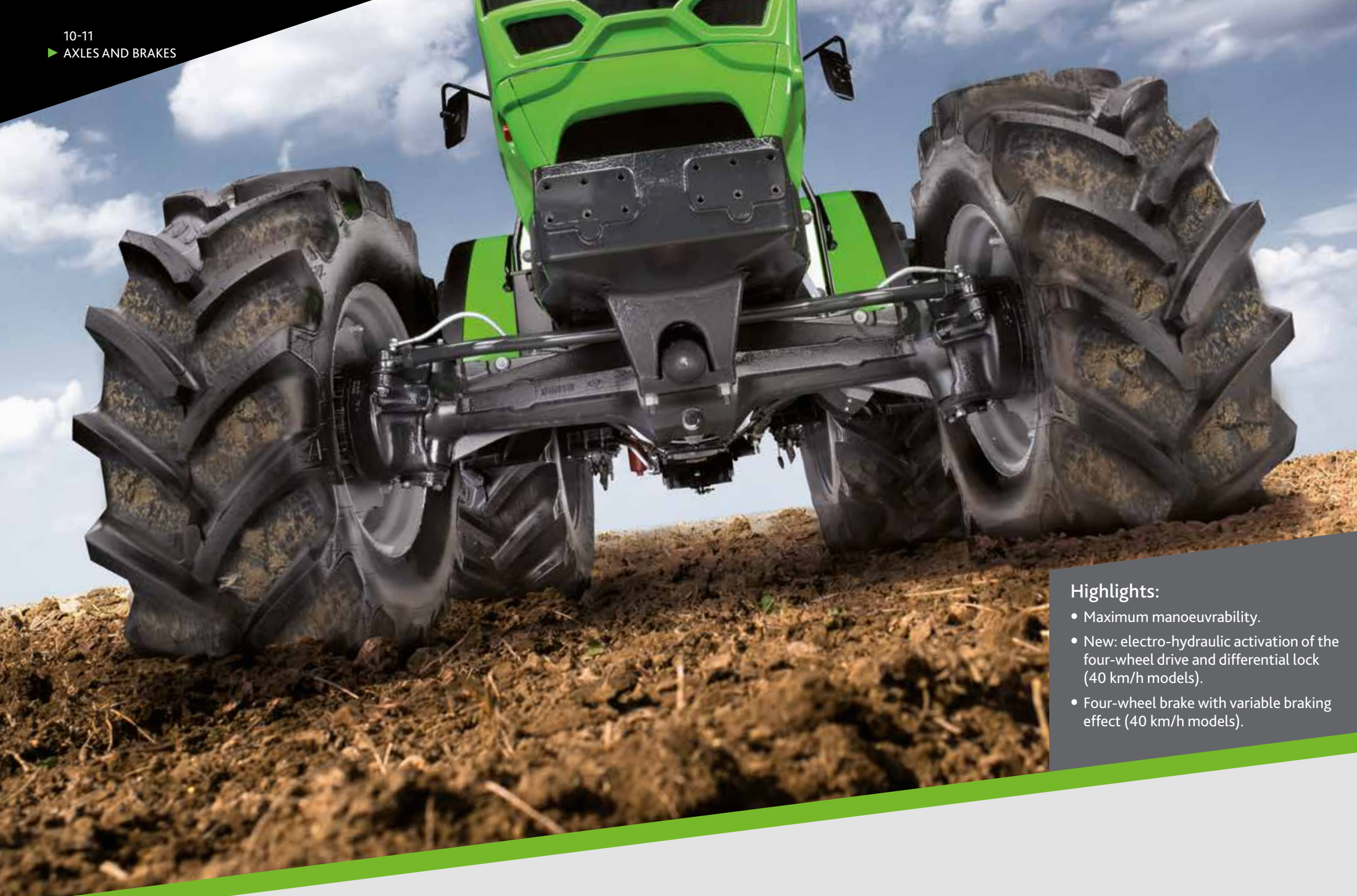
The compact bonnet allows a steering angle of up to 55°.
