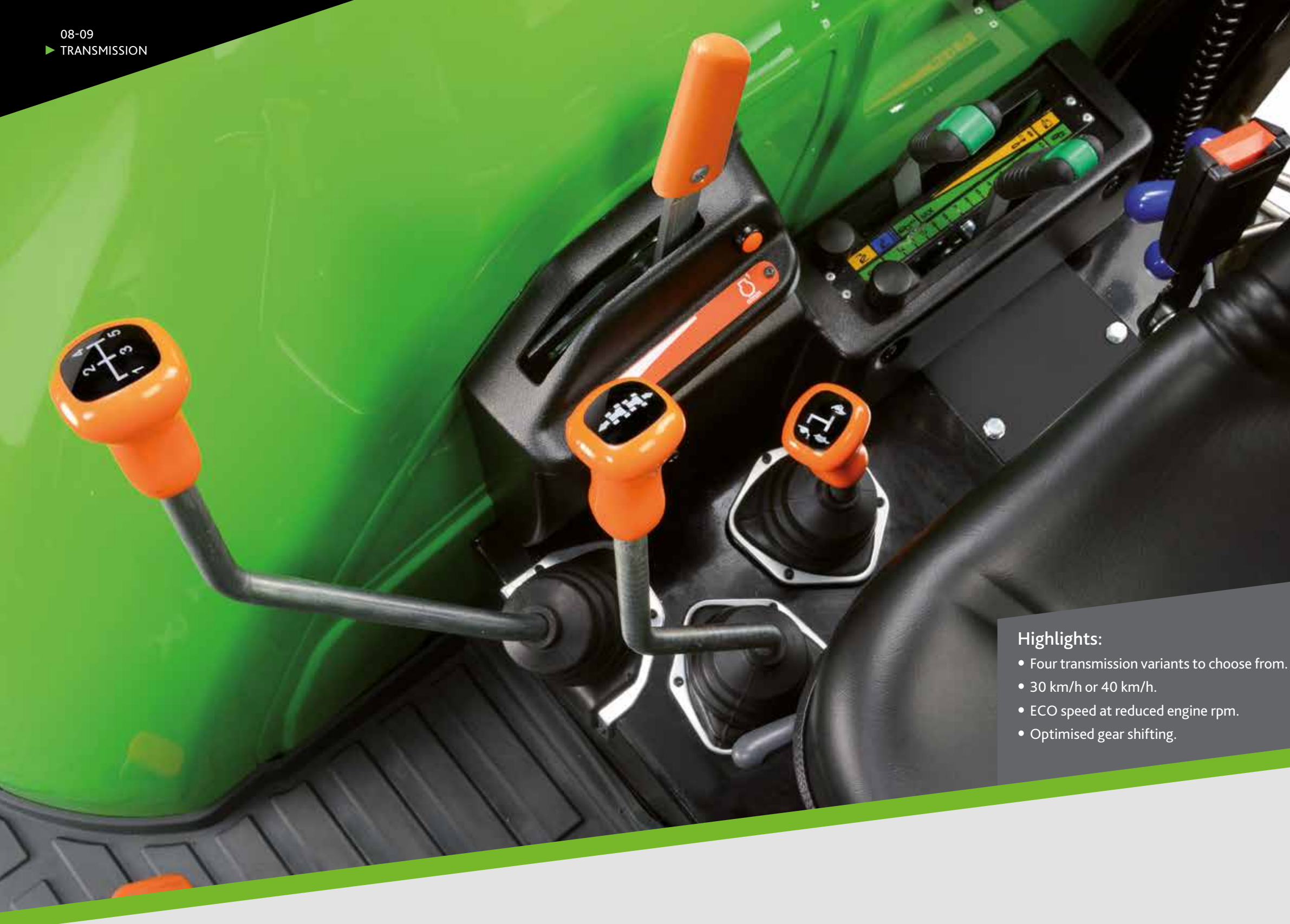
Finely graduated speed ranges from 8+8 speeds ...
