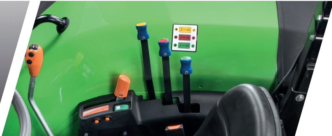
> Practical layout of spool valves control and EasyLift system.
