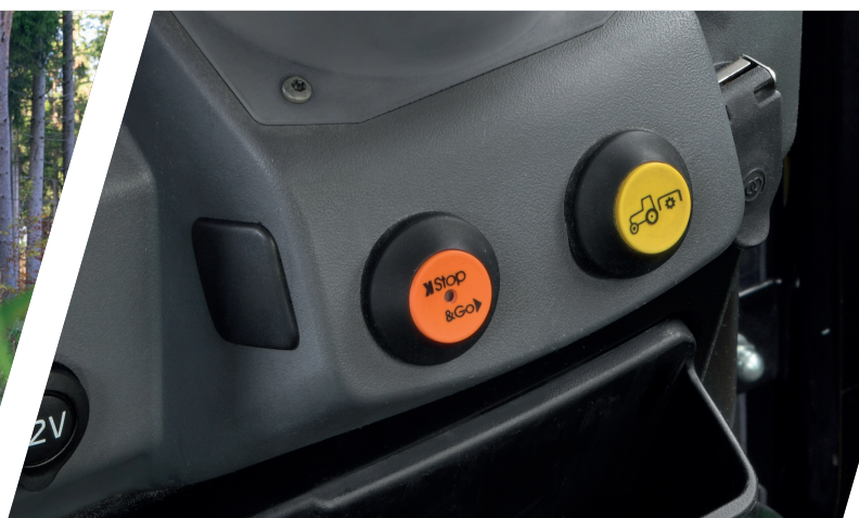
> Electro-Hydraulic PTO speed engagement on Models with PowerShuttle.
