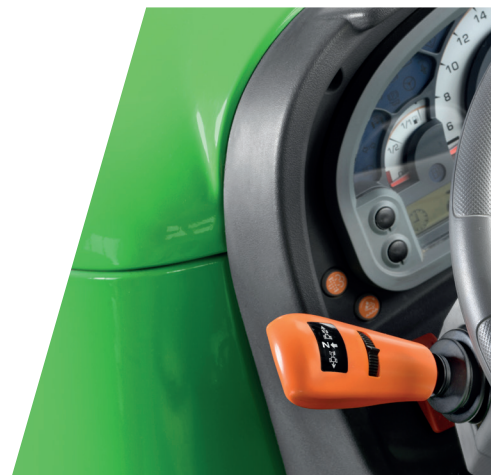
> Adjustable steering column and PowerShuttle.
