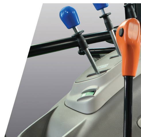
> 5-speeds knob with ComfortClutch button.
