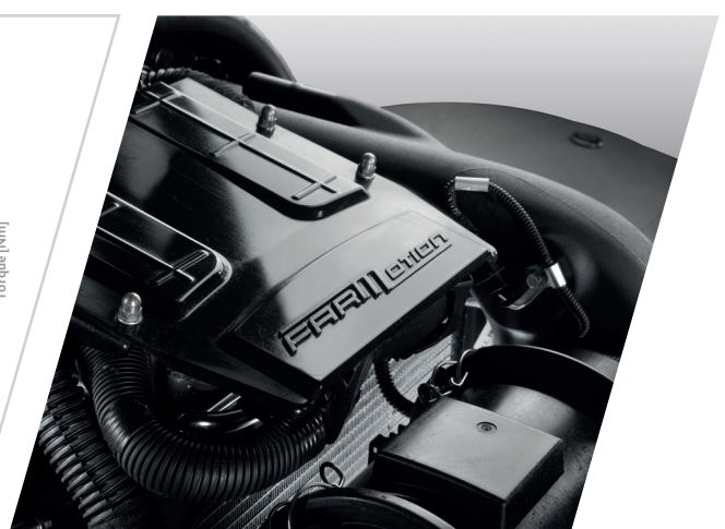
> EPA compliant FARMotion engines with Common Rail injection and power outputs up to 102 HP.
