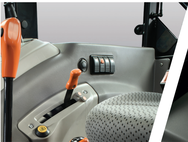
> PowerShuttle with SenseClutch.
