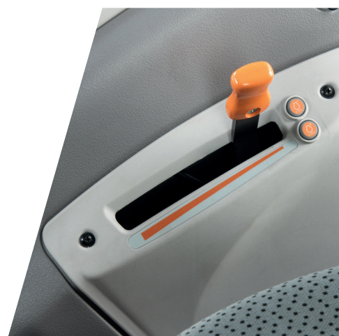
> Electronic hand throttle with two engine memory speeds..
