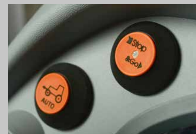
Stop&Go. Start and stop the vehicle in comfort without using the clutch pedal.
