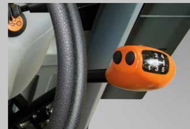
PowerShift. Change gears at the push of a button without depressing the clutch.
