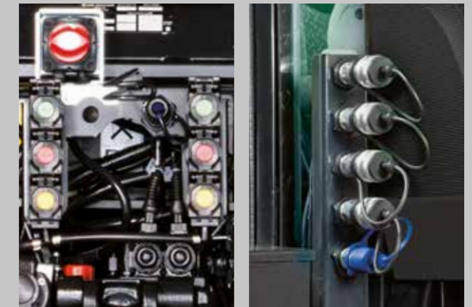
Up to six hydraulic spool valves at the rear and front.
