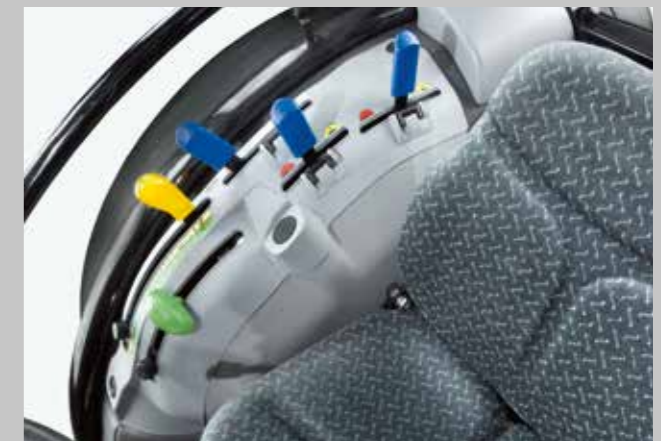
Mechanical rear lift levers, functional and ergonomic.
