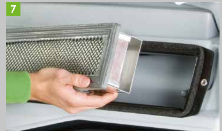
The cab air filter prevents dust and chemicals. Clean air inside the cab at all times.
