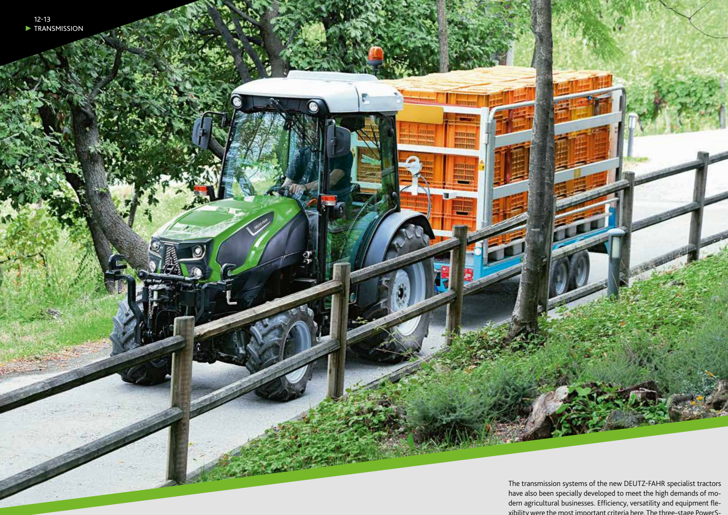
PowerShift. Change gears at the push of a button without depressing the clutch.
