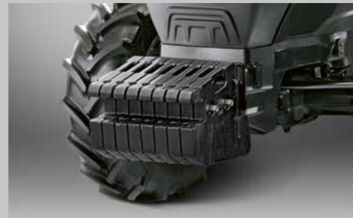
Different front weights for working with heavy rear attachments.
