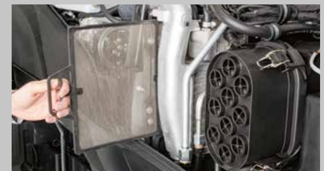
Engine efficiency is aided by the large, newly designed cooling package, improved air flow and the Powercore air filter.
