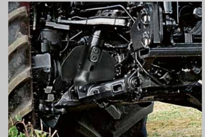
Independent wheel suspension with double wishbone design.
