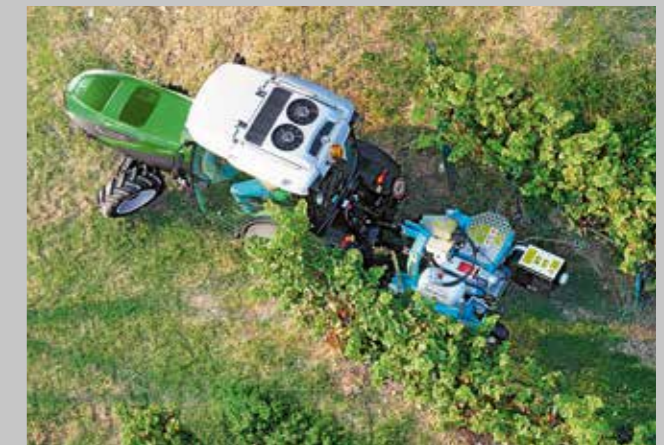
Improved turning radius thanks to a slimmer front support.
