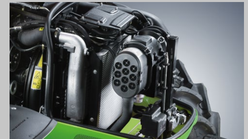
Compact radiator with Visco fan and PowerCore air filter for maximum engine efficiency.
