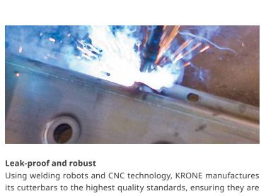
its cutterbars to the highest quality standards, ensuring they are fully welded and permanently lubricated. After all, the cutterbar is the heart of every disc mower.
