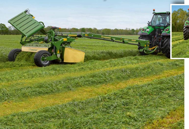
The EasyCut trailed mowers with a working width of 2.71 m to 3.60 m offer maximum flexibility and, thanks to their wide variety, meet the most diverse requirements worldwide. The TS models score on their compact design and the TC models on versatility. The central drawbar gives you the option of working to the right or left of the tractor. These trailed mowers are available either with tine conditioner or roller conditioner. All conditioner models can be equipped with the KRONE Collect system.
