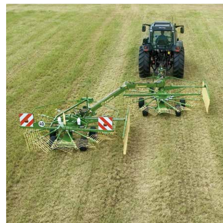
Swathing all material to the left, forming a twin swath
