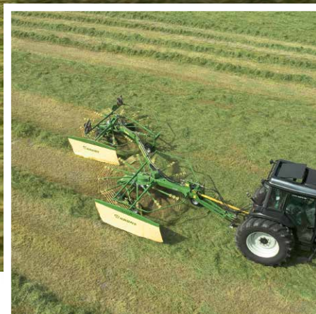
Forming a twin swath Raking 6.80 m into two swaths
