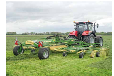
Swadro TC 1000 / 1000 Plus twin-rotor rake centre delivery Variable working widths from 8.90 m to 10.00 m
