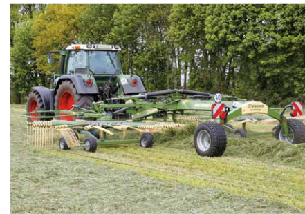
Swadro TC 930 / 930 Plus twin-rotor rake centre delivery Variable working widths from 8.10 m to 9.30 m
