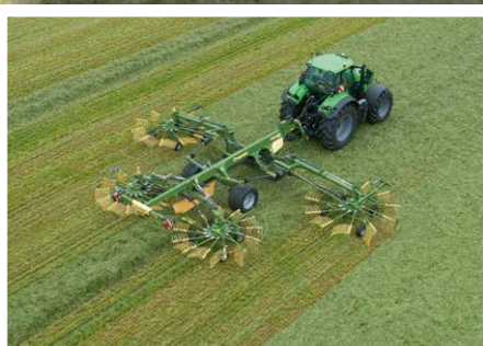
Swadro TC 1250 / 1250 Plus four-rotor rake centre delivery Variable working widths from 9.80 m to 12.50 m
