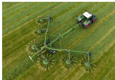
Swadro TC 2000 Six-rotor rake centre delivery Variable working widths from 10.00 m to 19.00 m
