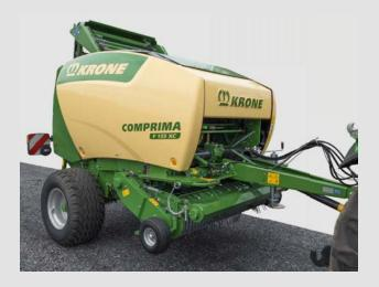
vice – thanks to their uncluttered build and design. It can unload bales of different diameters and compacts from the outside to the inside; with larger bale diameters, it leaves only a very small soft core. Thus, it achieves high bale weights.
