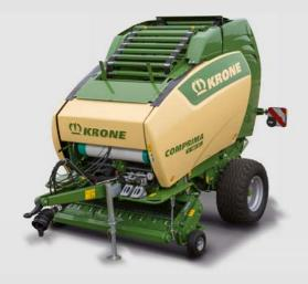
are set to handle all crops and conditions. Smaller bale sizes are often preferred in grass silage whereas larger bales are more typical in hay and straw. Depending on the crop, the baling density in the core of the bale can be reduced, which is perfect for ventilating hay bales.
