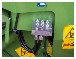
The lubrication manifolds All grease points are grouped into easy-access grease banks, saving time and increasing the operator comfort.
