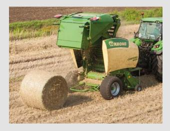
The semi-variable round baler Comprima F 155 (XC) The Comprima F 155 can roll bales of a diameter between 1.25 m and 1.50 m. Operators simply set the required diameter in 5 cm increments on an easy-to-use system. Thus, the machine combines many advantages of fixed and variable chamber balers. They are also very cost-effective and exceptionally easy to operate and ser-
