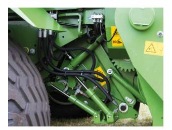
**The hydraulic blade group control system** The optional hydraulic blade group control system is operated from the tractor seat, hence saving valuable time.
