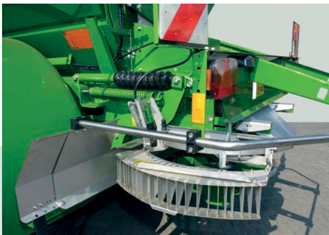
Limiter border spreading system in working position
