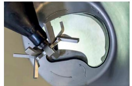
Stage 3: Hopper aperture wide open
