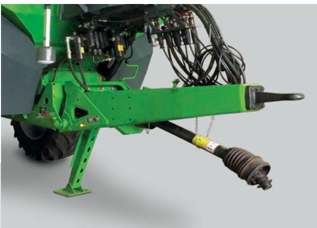
✓ Clevis type coupling with towing eye
