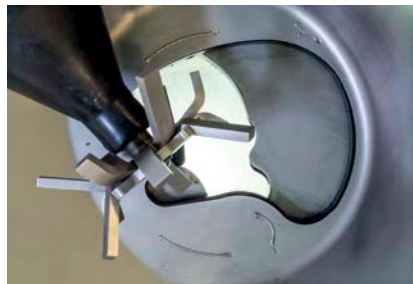
Stage 2: Hopper aperture half open
