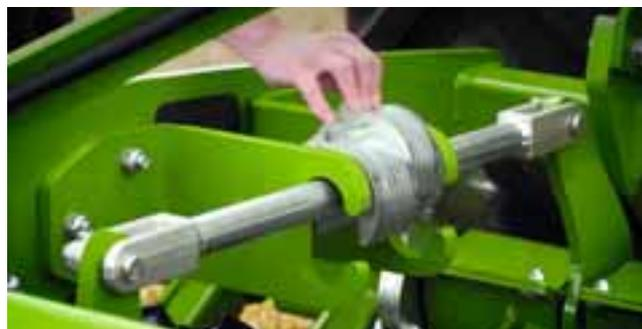
✔ Working depth adjustment via spacers – here at a mid-working depth
