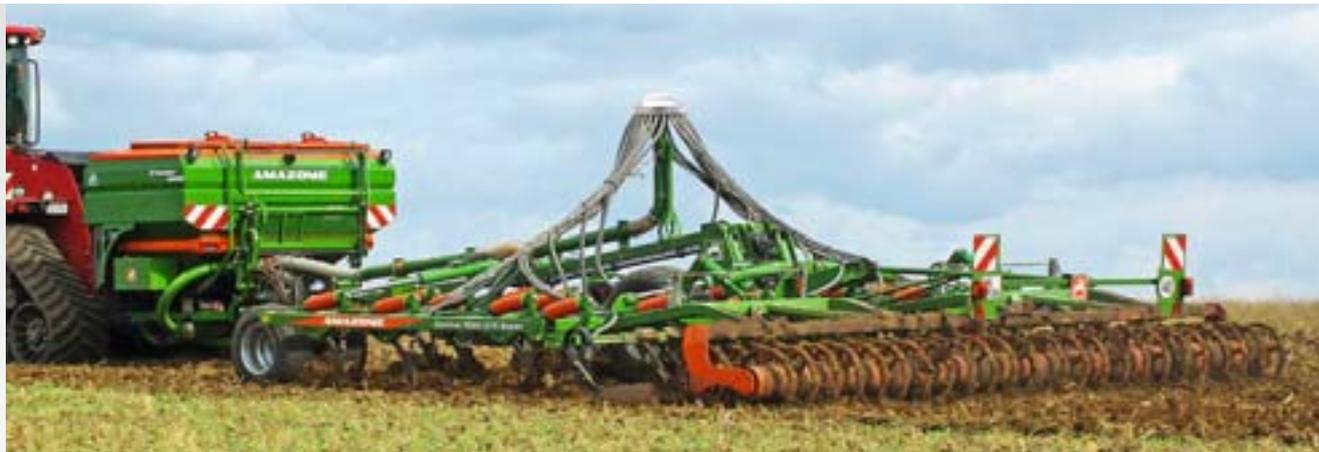
XTender 4200 with Cenius 6003-2TX and conveying system for fertiliser application
