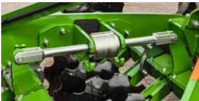
✔ Working depth adjustment via spacers – here at a shallow working depth
