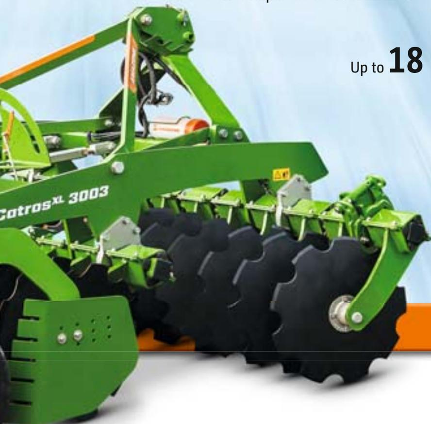
Due to its open frame design and the large through passage potential, the Catros<sup>XL</sup> compact disc harrow is optimally suited to farms with much organic matter. Due to the large diameter, fine or coarse serrated, 610 mm discs, working depths down to 16 cm are no problem. In working widths of 3 m to 4 m and operational speeds of 12 to 18 km/h, high acreage outputs with an excellent quality of work can be achieved.
