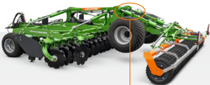
Hydraulic top tie bar on Certos 6002-2TX
