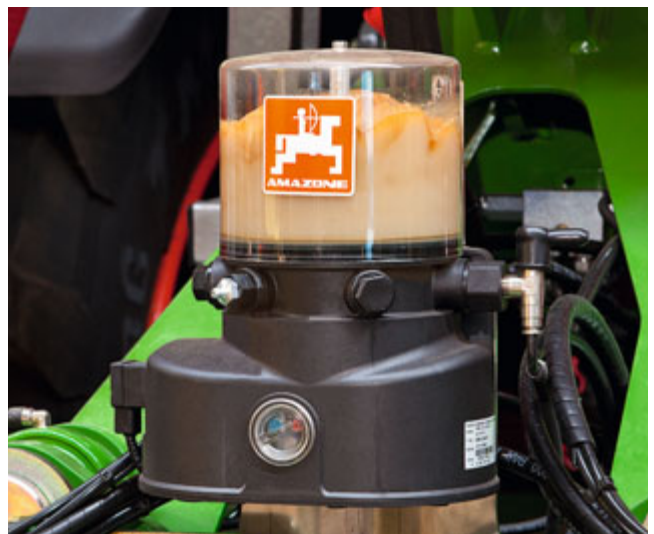
Pump with reservoir
