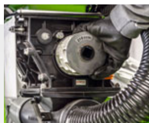
Easy exchange of the metering rollers
