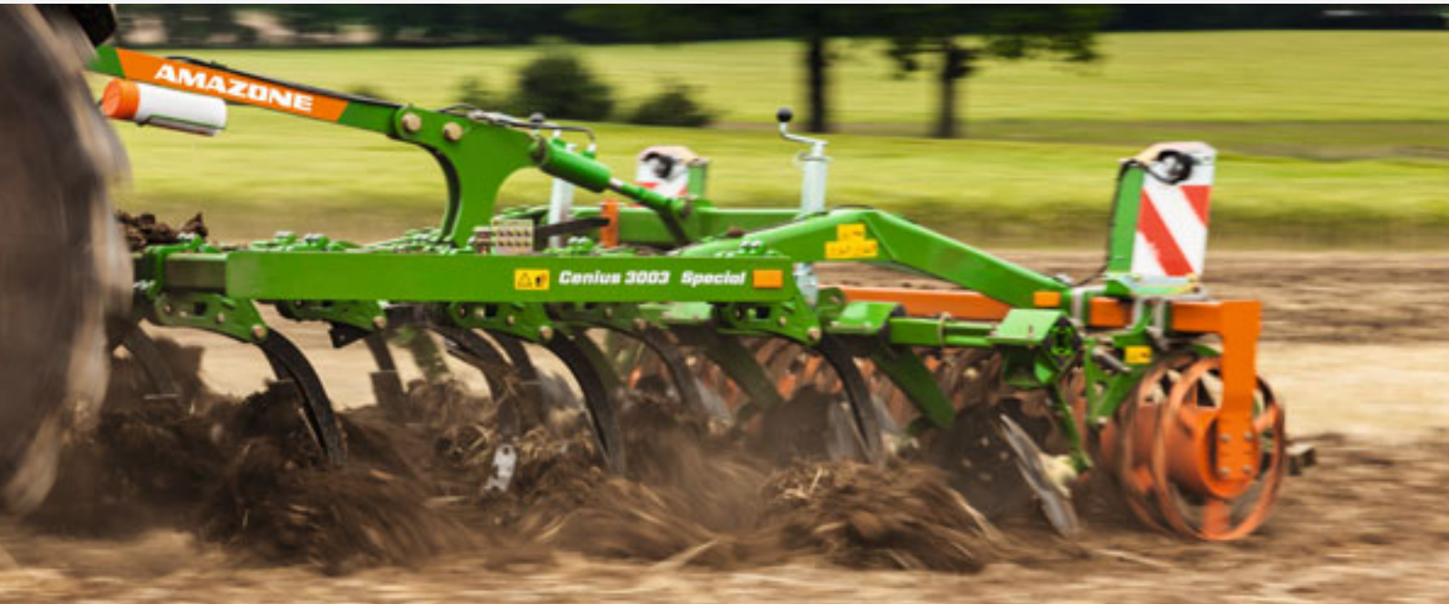
Cenius 3003 Special with C-Mix Special tines
