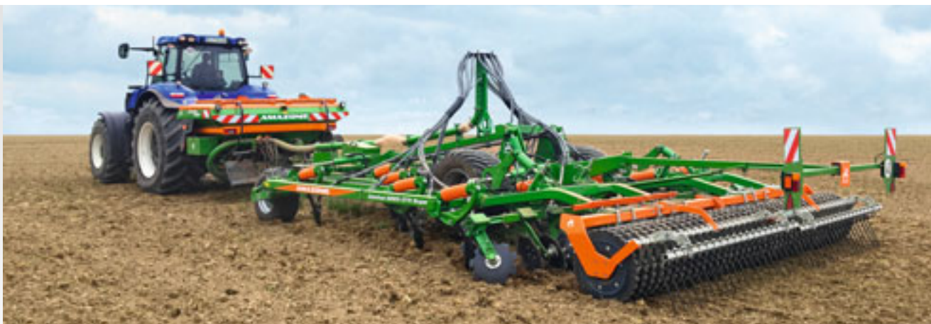
XTender 2200 with Cenius 5003-2TX and conveyor system for fertiliser application
