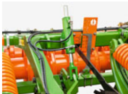
Hydraulic cylinder for setting the depth of the levelling section
