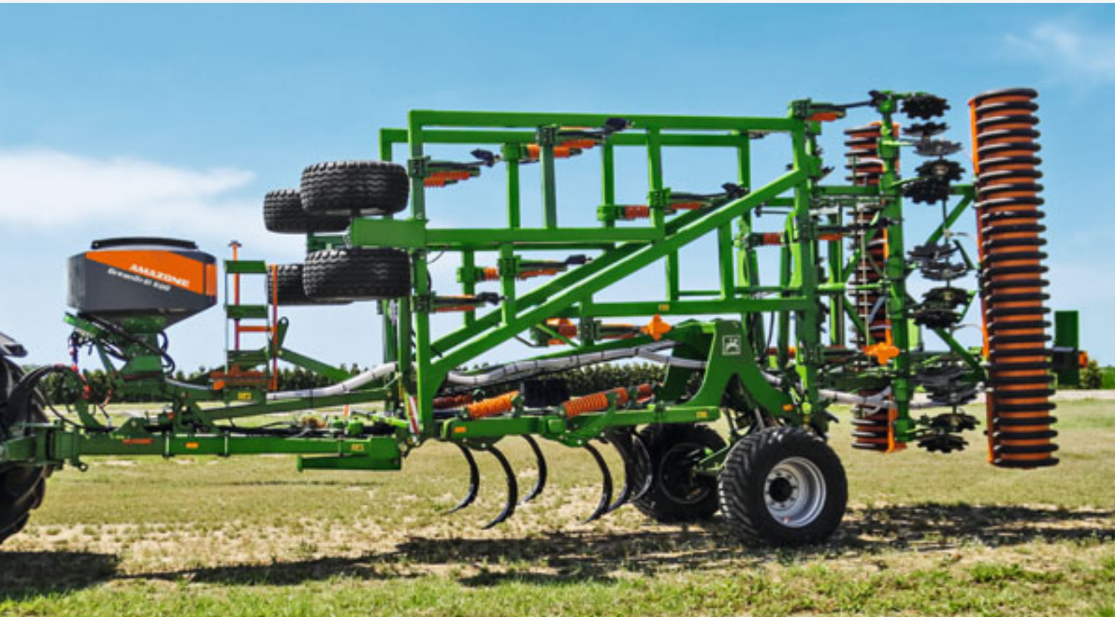
Cenius 7003-2TX Super with GreenDrill 500 seeder box
