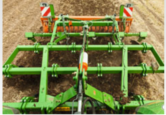
3-stagger frame mounting on the Cenius 3003 Special
