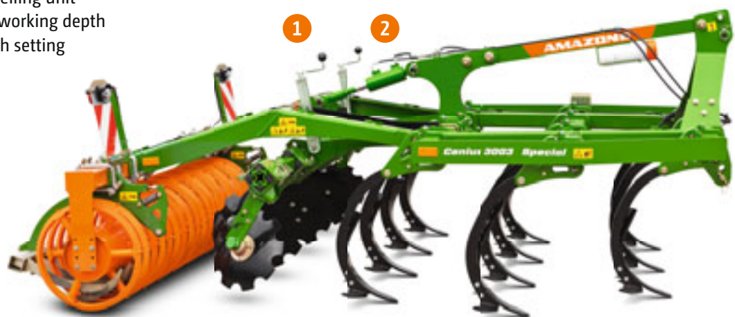
Cenius Special: C-Mix tines with shear bolt overload safety device and Angle profile roller
