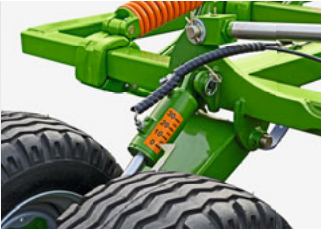
Setting scale for the hydraulic tine section depth adjustment
