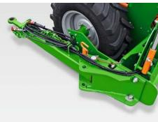
The drawbar for road transport is folded in when sowing
