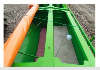
The rear part of the hopper can be utilised for fertiliser.
