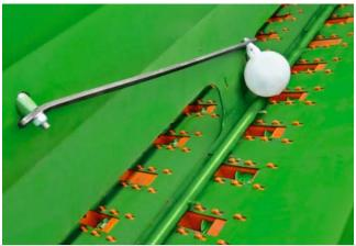
Via the removal of the partitions and closing off the fertiliser metering system, the complete hopper volume can be utilised for seed.
