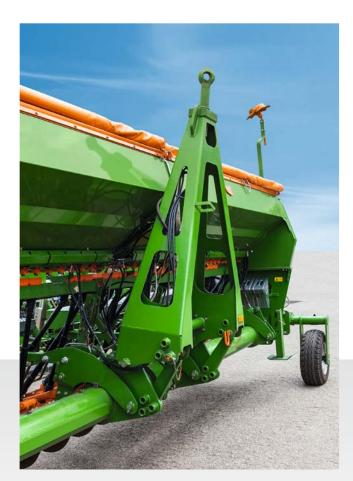
Hydraulically-folding transport drawbar
