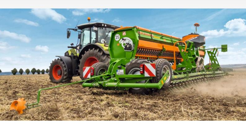
The D9 "Combi" with a working width of 6 m has established itself successfully in the Russian market and is perfectly suited for mounting onto smaller tractors with little lifting power.
