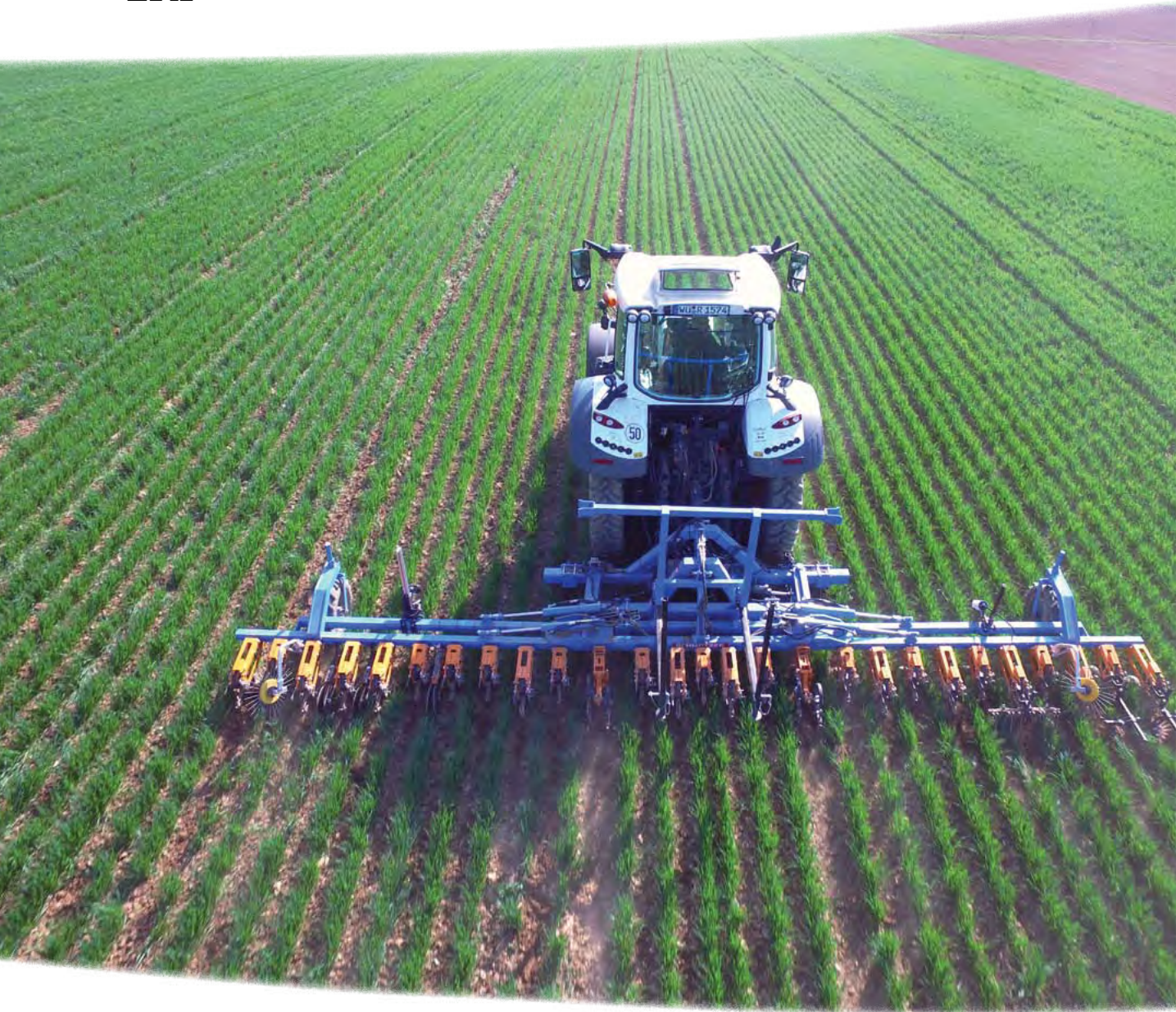
Grain hoe with EKP long and EKP short, the tyre track is processed by MPPs
