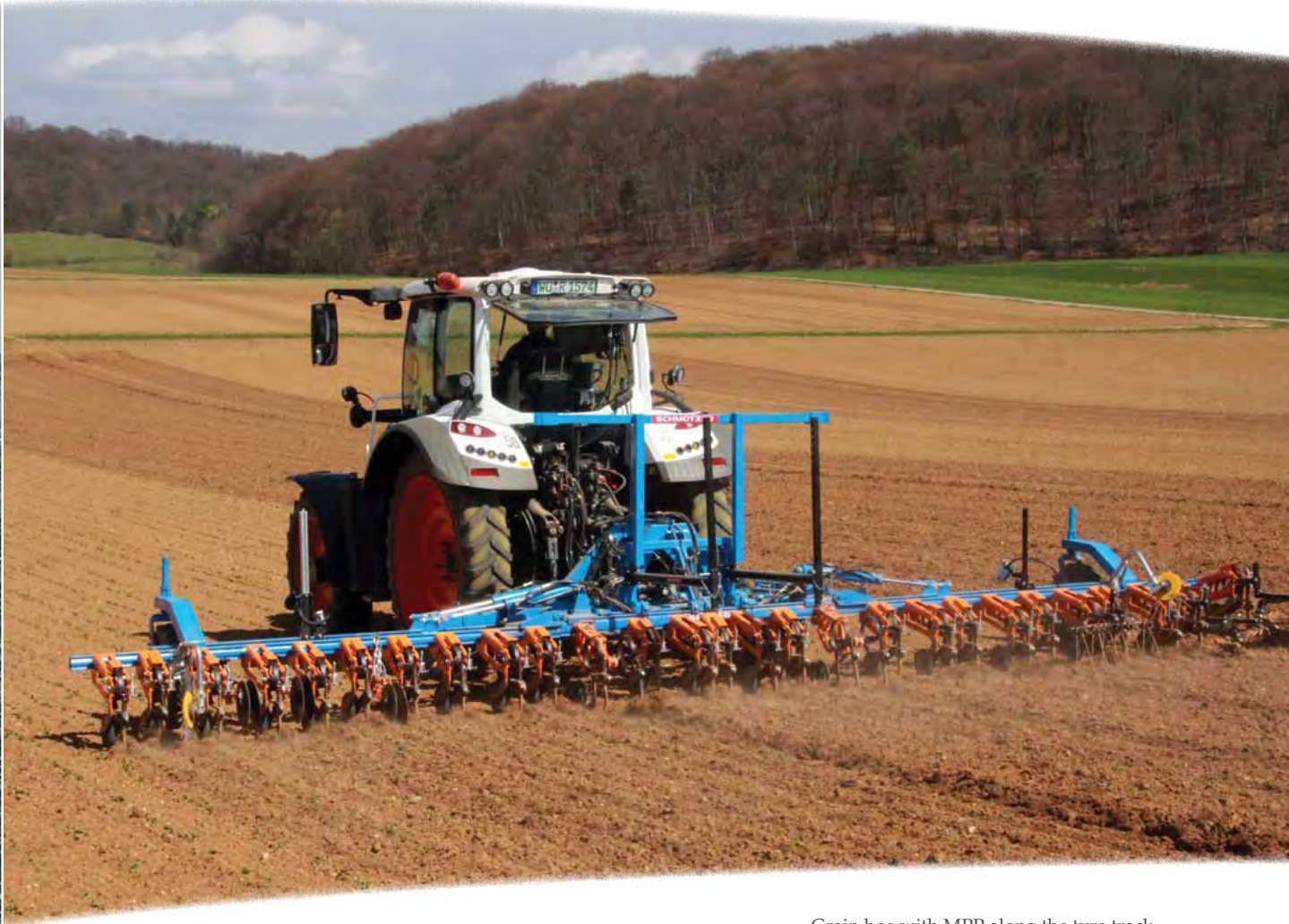
Grain hoe with MPP along the tyre track
