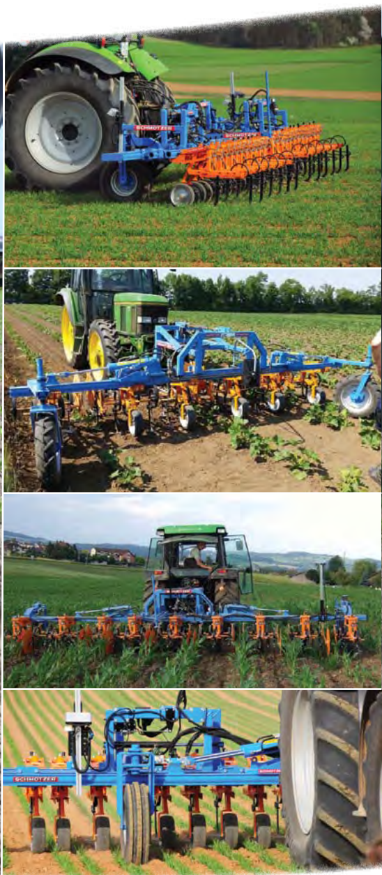
30 row cereal hoe in Frankonia 3 row hoe for cucumbre in Austria 8 row hoe for corn with camera in Switzerland
