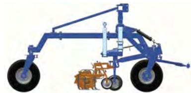
System of wheels with bolts in the direction of travel, for road use and fieldwork
