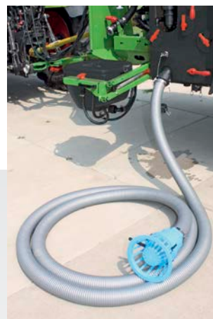
Filling via the suction hose
