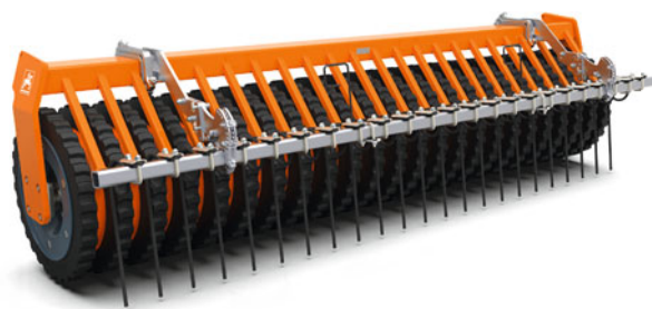
Harrow system for KWM & DW following rollers
