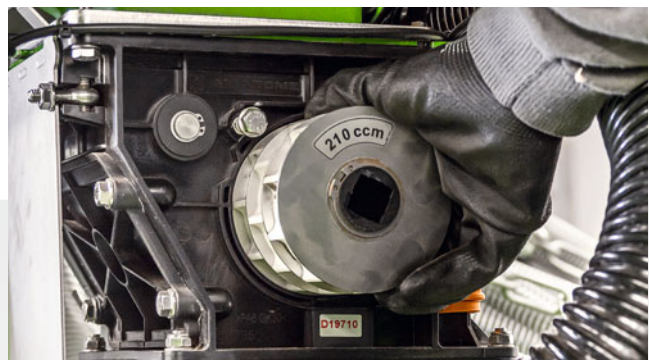
Easy exchange of the metering rollers
