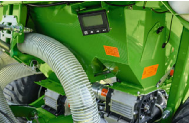
Primera DMC with electric metering drive and TwinTerminal 3.0
