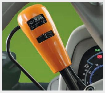
PowerShuttle with Sense Clutch and five adjustment levels.
