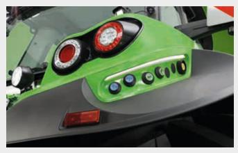
▲ Illuminated push buttons for external control of the rear lift, the PTO and a spool
