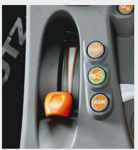
Independent hand throttle and electrohydraulic activation of differential lock, four-wheel drive and ASM function.
