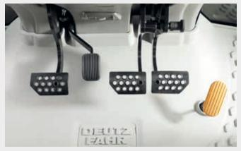
Pedal layout with Engine brake<sup>PLUS</sup> (Pedal between clutch and brake pedals).
