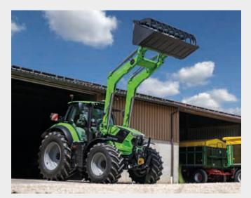
Maximum lifting height of 4.5 m and a breakout force of 3770 daN.
