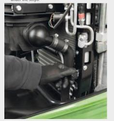
Cooling package with easy opening mechanism.
