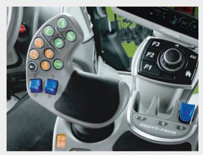
Ergonomic MaxCom joystick with lift buttons, engine and transmission control, headland management button and two proportional hydraulic valve control units.
