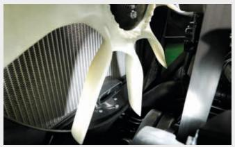
Electronic viscostatic fan (eVisco) with suction hose for the air filter pre-cleaning system (removes 95% of coarse particles before they can reach filters).
