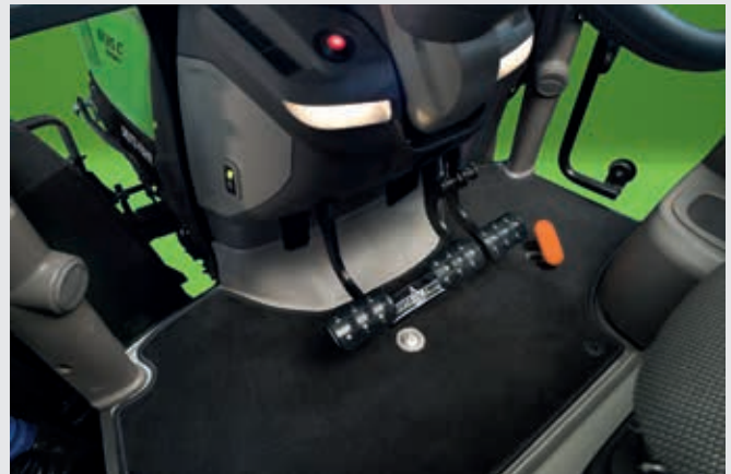
↑ Hydraulic Engine Brake activation.
