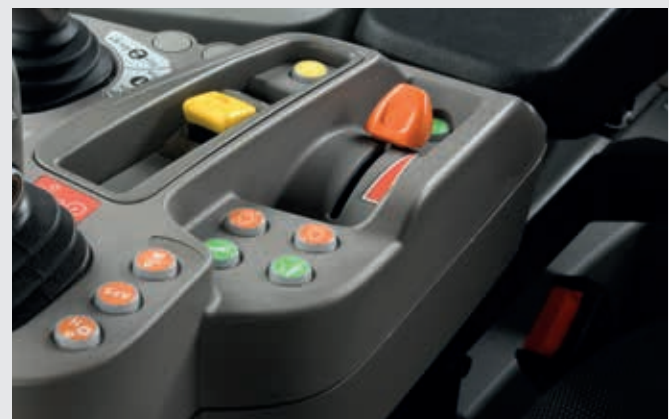
Electronic hand throttle with 2 engine memory speeds.
