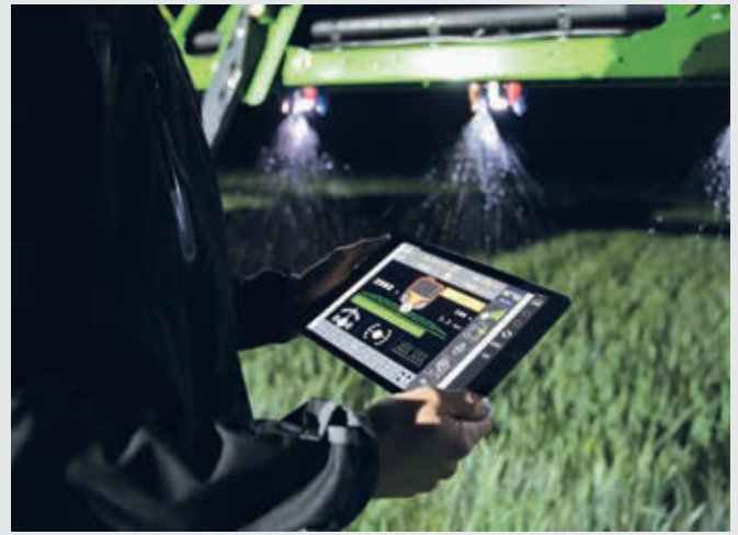
↑ XTEND function with tablet, control of implements via ISOBUS UT while being outside of the cab.
