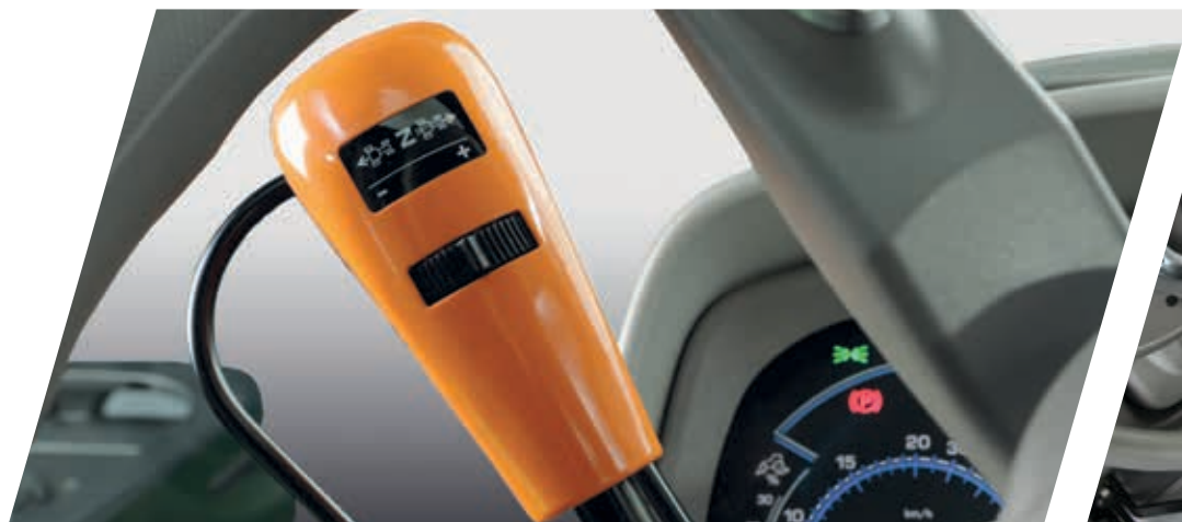
> PowerShuttle with Sense Clutch and five direction change settings.
