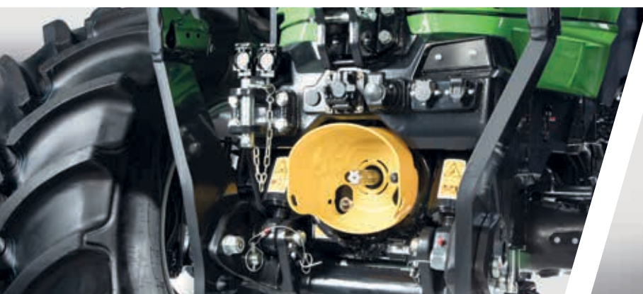
> Front lift with 5450 kg lifting capacity and DualSpeed front PTO.
