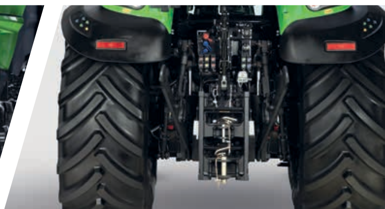
> Rear linkage, five rear spool valves, external controls on fenders on both sides.
