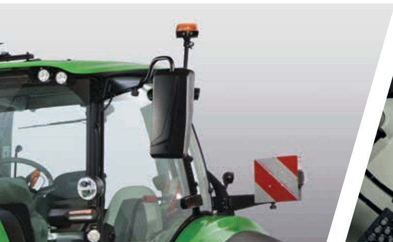
> The XLargeVision mirrors and the internal visibility package improve the 360 degree view significantly.
