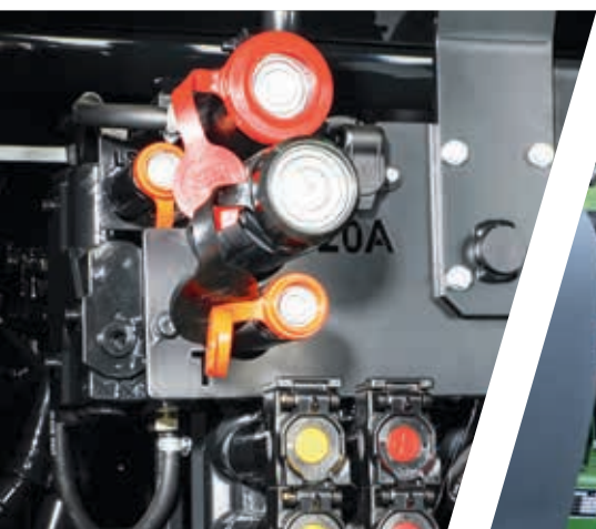
> Power Beyond with flat face couplers for a clean connection.
