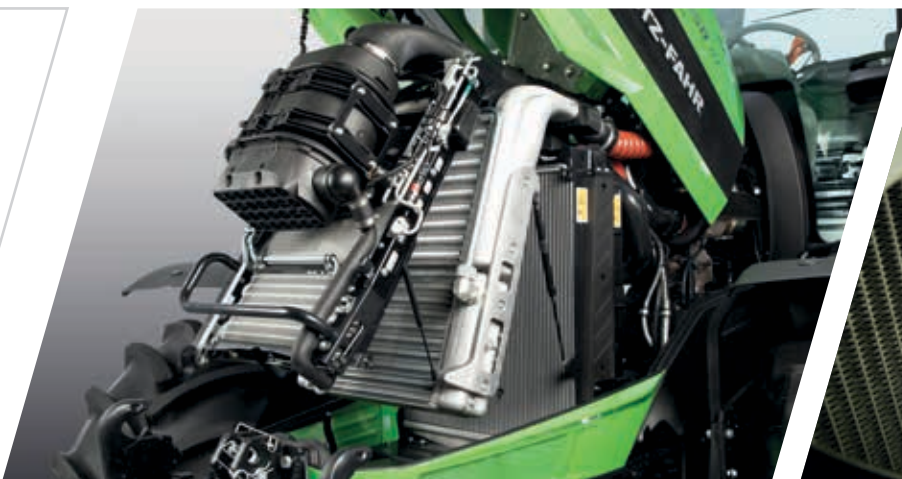
> Aluminium cooling system with with one-hand access lever and Powercore air filter.
