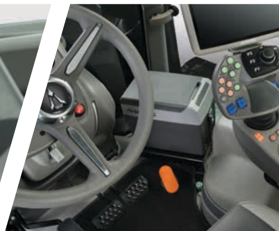
> Ergonomic MaxCom joystick with front and rear lift, engine, transmission, headland management and two proportional hydraulic valve control units.
