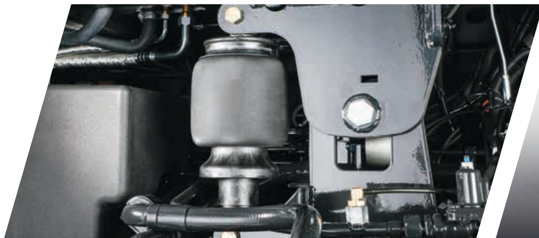
> Air-suspended cabin for maximum driving comfort.
