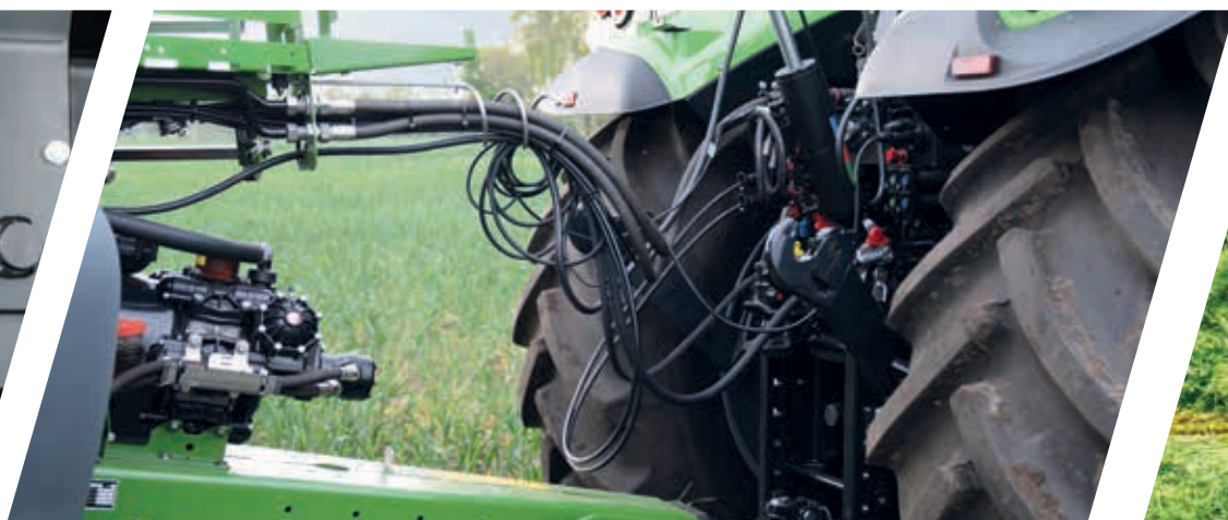
> Rear linkage in transport position for less interference with drawbars while cornering.
