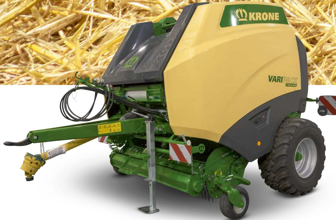
**Camless EasyFlow pick-up with chevron-lined tines**
