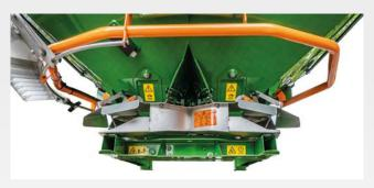
Row spreading attachment directly behind the spreading discs
