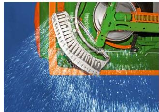
The Limiter can be hydraulically folded up out of the spread fan from the tractor seat.
