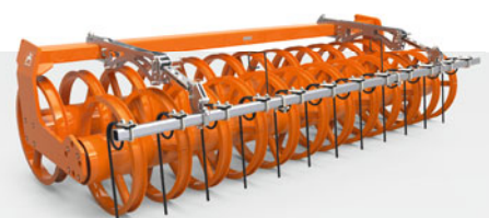
Harrow system for DUW following roller
