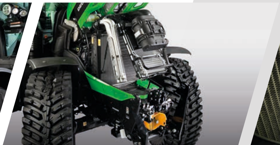
> Aluminium cooling system Performance Pro with one-hand release lever for models 6210-6230.
