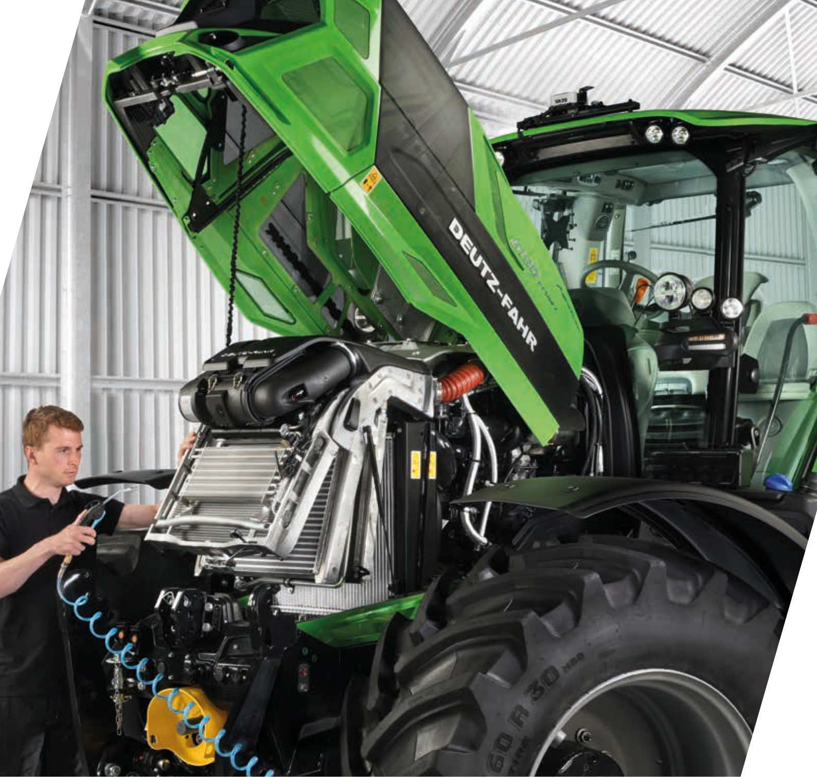
> Easy access to radiator package and air hose and air gun integrated for quick cleaning.
