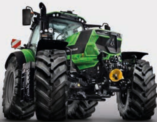
> Front suspended axle with 100% front differential lock.
