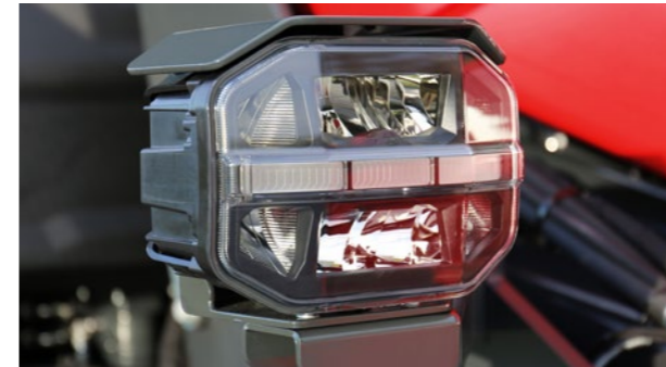
The driving headlights are equipped with LEDs and daytime running light.
