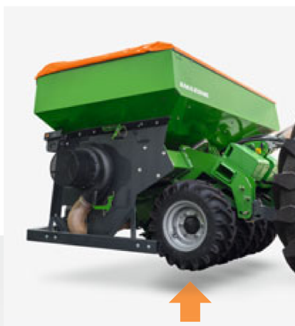
FTender with T-Pack F front tyre packer in the transport position
