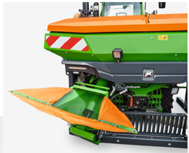
A filling auger with a folding reception hopper is available as an option. This allows easy filling directly from the trailer. The filling auger is securely closed with a lid in the transport position.
