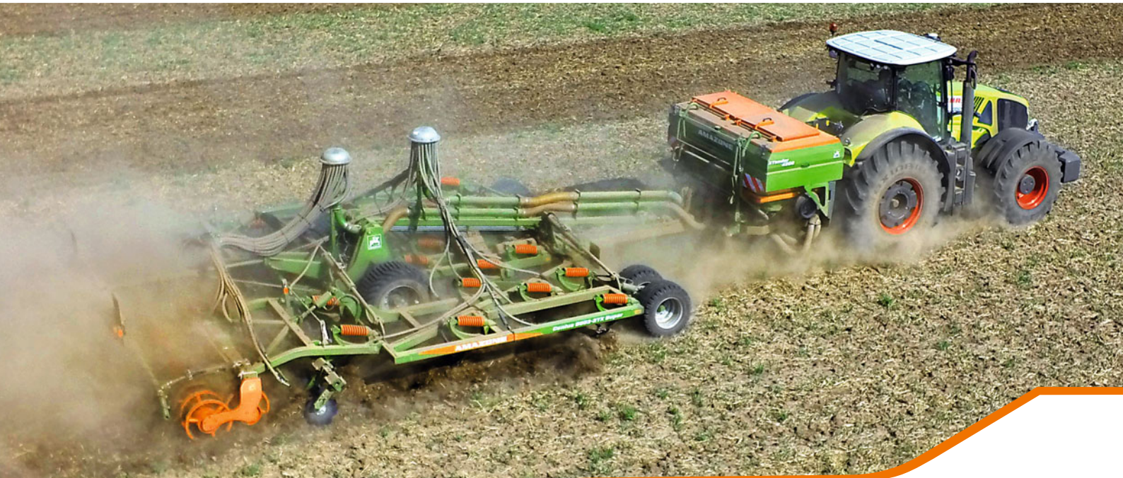
XTender 4200 in combination with Cenius 6003-2TX and twin conveying systems for delivering fertiliser and seed
