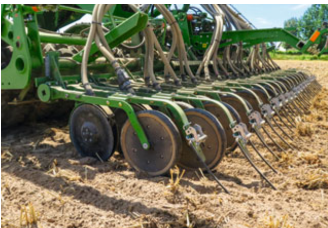
TwinTeC plus coulters with hydraulic coulters pressure regulation
