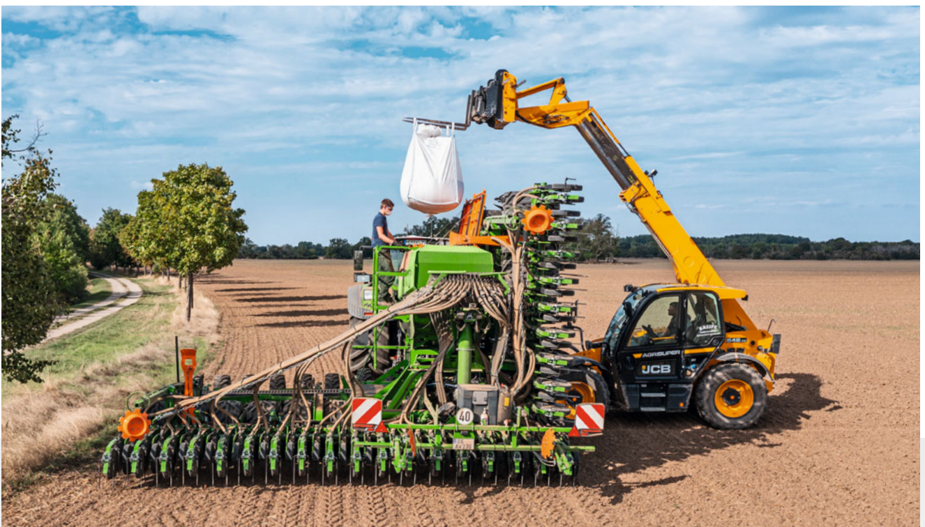
Half-side folding during loading considerably reduces the loading reach and also allows the machine to be filled via smaller telescopic loaders
