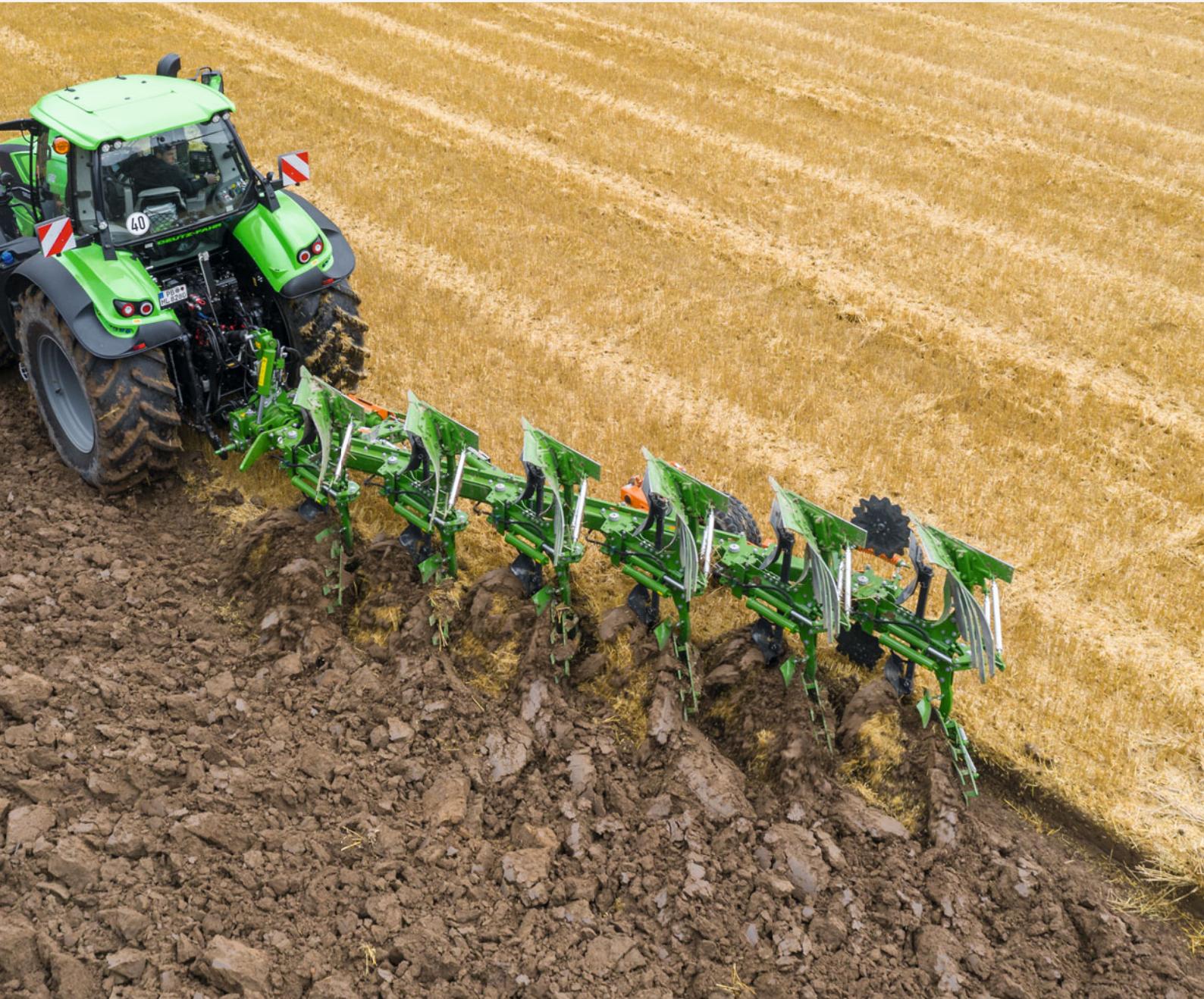
Teres 300 VS with 6 furrows for comfortable ploughing at maximum working speed
